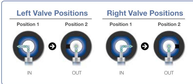
**Note:** The left and right valves can move independently of each other, as indicated in the diagram above.
